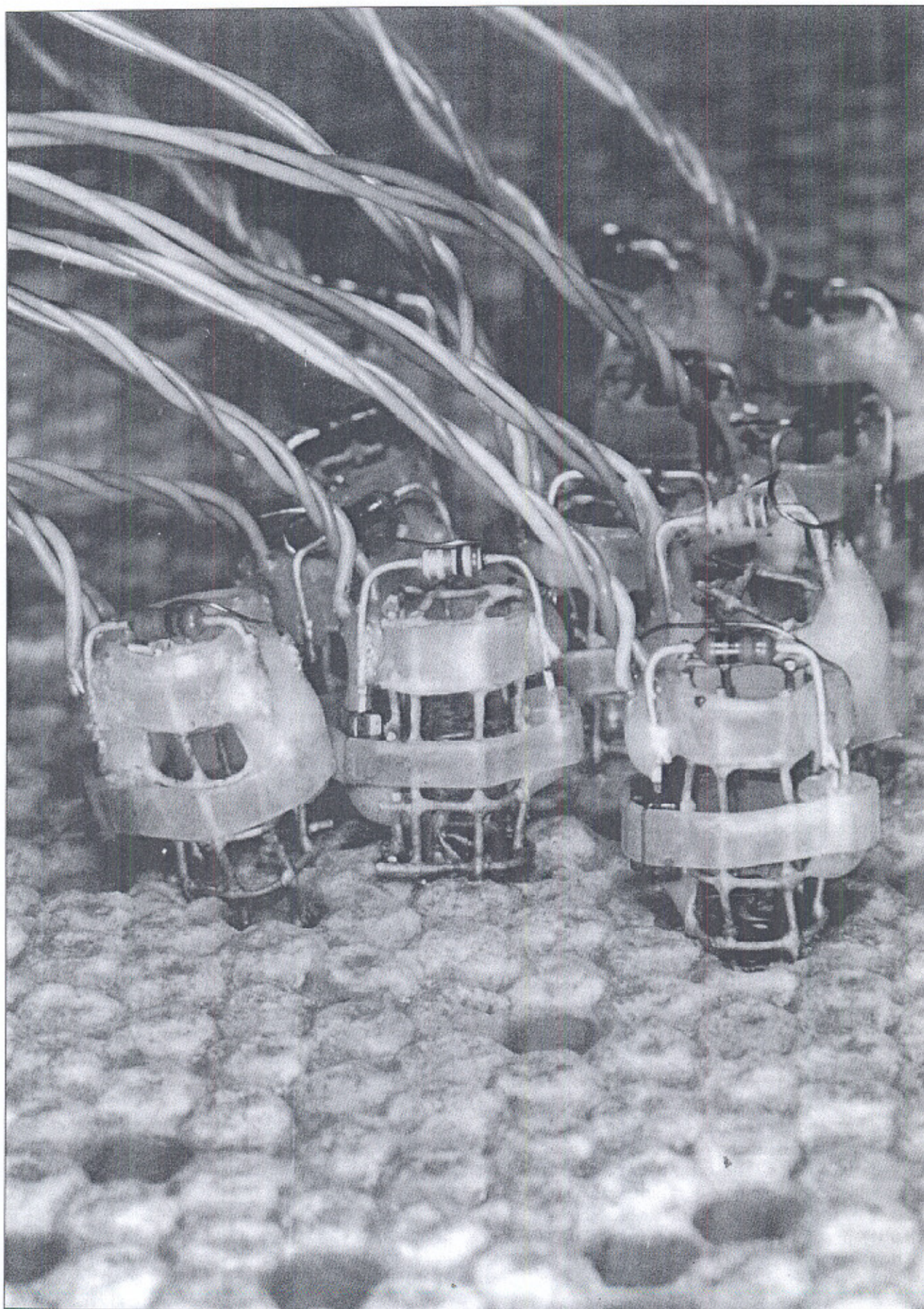
FIG. 1. Infra-red barrier system used to measure the time of emergence of worker honey bees.
