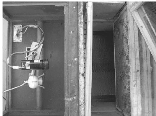
Fig. 1. Experimental setup from left to right: camera, illumination frame, comb
