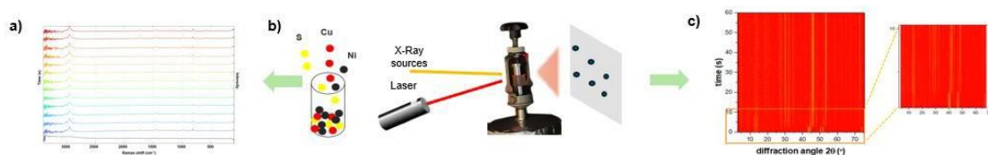
Fig. 1 Tandem time-resolved in situ monitoring of mechanochemical treatment of Ni:Cu:S 1:1:2 system: a) Raman spectra, b) scheme of experimental setup, c) XRD patterns heat map.
